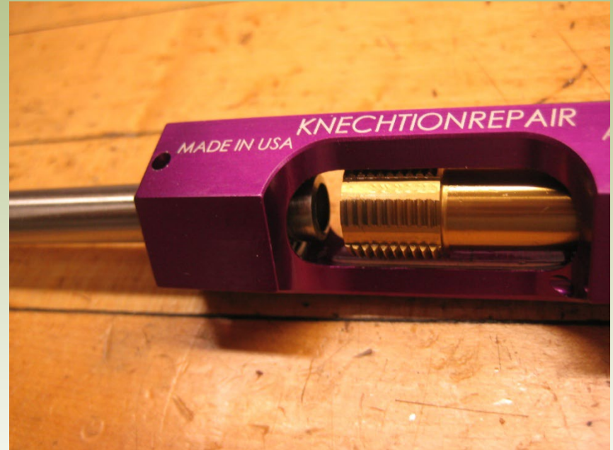
All Nuts with a Thread or Threads Removed were Tapped Following Turning using The KnechtionRepair 3/8-Inch Tap Kit
