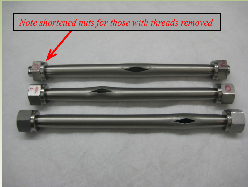
Test Articles Following Tube Burst Failure at 15,000 psig ( \pm 200 psig)
